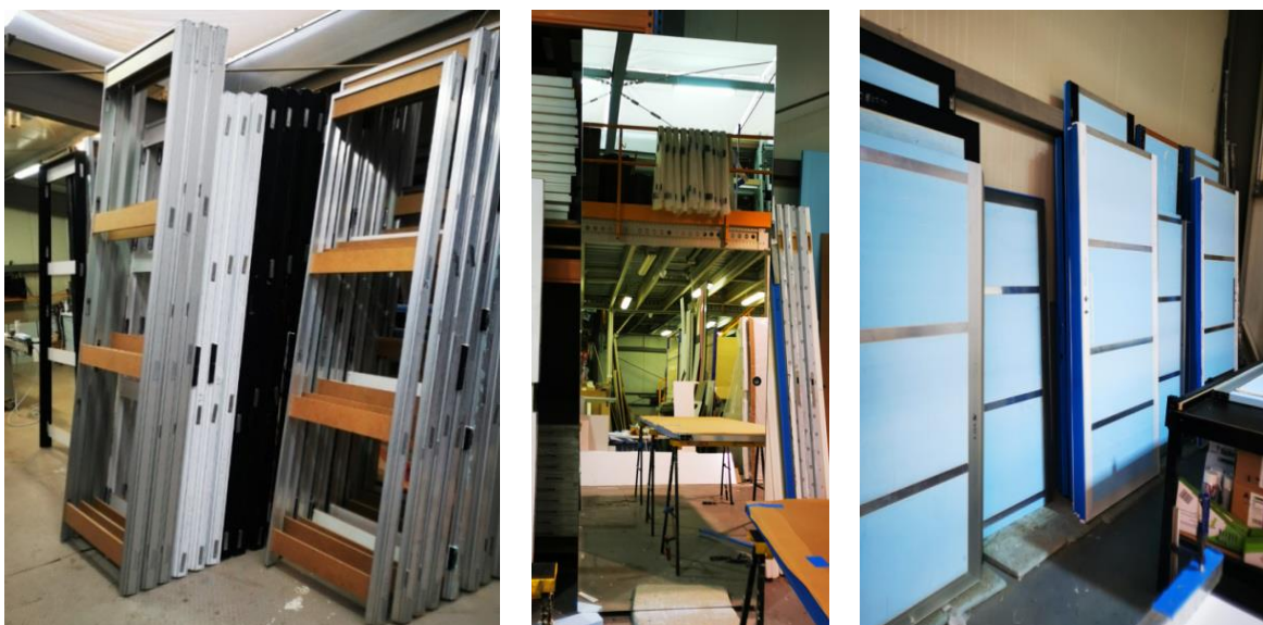
Figure 2. Photos of door frames and leaves at different stages of finishing, with different finishing materials, while verifying the possibility of manufacturing in various extreme and intermediate dimensions. Source: Photos from the archives of the Zeromur company
