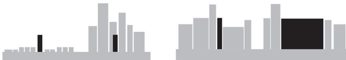
Fig. 1. Illustration of the problem of the relative height and size of a building in the context of adjacent buildings (a) context (b) proportion. Source: CTBUH, 2013-2022
