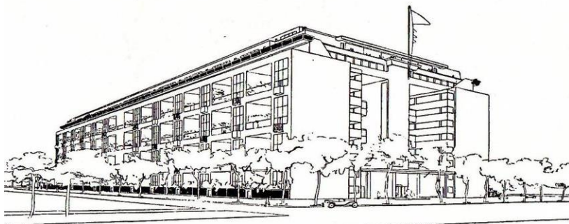
Fig. 1. Studies on residential architecture by Le Corbusier from the 1920s. The author envisioned creating large loggias within the structure of the building, compensating residents for the lack of direct contact with the ground. Source: Hilberseimer L., Grosstadt Architektur, Stuttgart, 1927.
