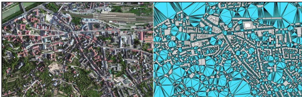
Fig. 2. Comparison of the same part of the city of Przemyśl (PL) represented by virtual city model embedded in popular open-access application Google Maps and by the N3D model of open spaces generated within LOD1 virtual city model. Source: Google Maps / author
