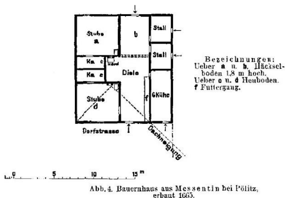
Fig. 10. Plan of the house in Mścięcino from 1665, as drawn by Lutsch. Description: over the spaces a and b loft for chaff with a height of 1.8 m., over the spaces c and d hayloft, f feeding cows. Source: (Lutsch H. 1887)
