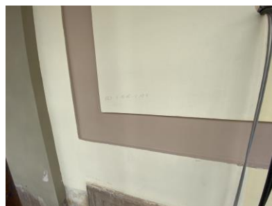
Fig. 5. Further color application trials prepared for evaluation by the heritage conservator. Source: by author
