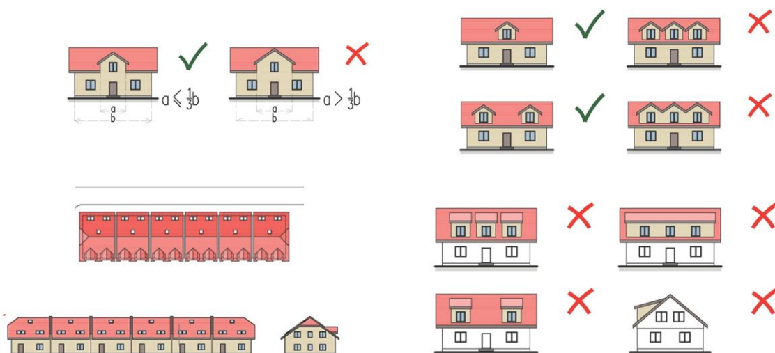
Fig. 6. Selected restrictions on shaping the building's shape and location in the field. Source: Środulska -Wielgus J. et al. 2020, by authors.
