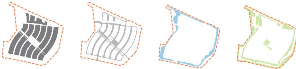
Fig. 20. Dronten. List of spatial structure elements: Analyzed area 37.6 ha, Built-up areas: 16.5 ha - 44%, Communication: 7.7 ha - 20%, Water: 4.6 ha - 12%, Green: 8.8 ha - 24% Source: author
