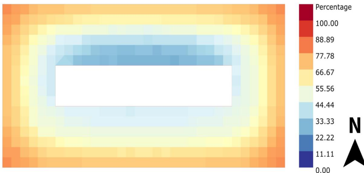
Fig. 1 Annual percent insolation results for a layout with parameters H=3.5m and D = 7.0m obtained in Grasshopper with Daysim software. The results show the percentage insolation time of one 1x1 [m] field with a minimum intensity of 500 lx during the hours of the analysis. Source: Original work, 2021
