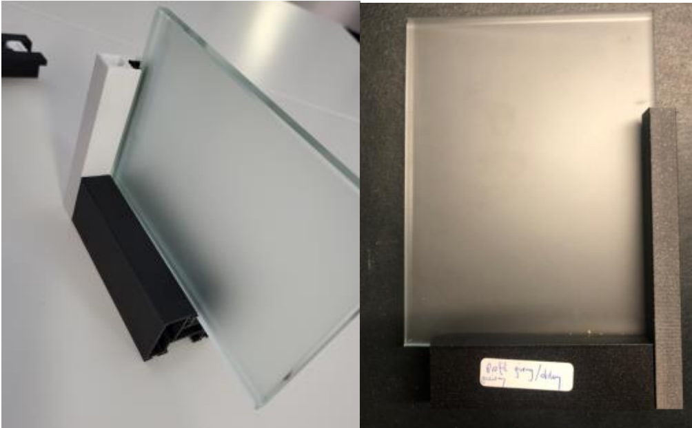
Fig. 2 3D prints of the glass system profiles with inserted glass panels – assessing the compatibility of profiles, glass sealing systems for 6 mm and 8 mm versions (also as a component printed from a flexible material using a special 3D technique) along with the node – corner connector. Source: Photos from the collection of PIU Design
