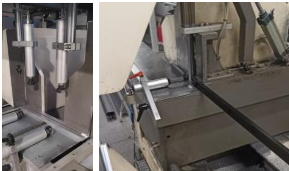
Fig. 4 Photos showing profiles during cutting on double-head saws. Specified cutting accuracies were achieved. Source: Photos from the collection of PIU Design
