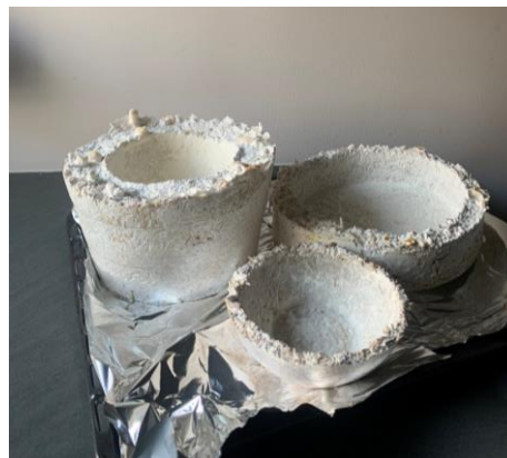
Fig. 1. Prototypes of flowerpots and bowls made with mycelium by Anna Lewandowska, source: photo by author
