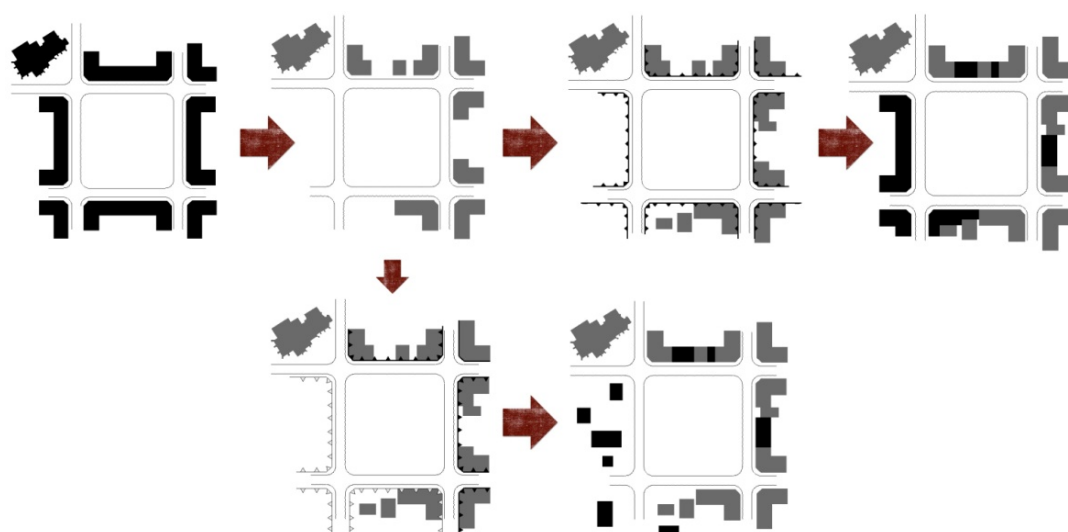
Fig.1 Effects of using the designated building line and building restriction line in shaping the walls of urban interior with numerous cavities. The designated building line offers an opportunity to preserve continuity of the structure. The use of building restriction building line may lead to irreversible loss of the interior's clarity and coherence (own scheme)
