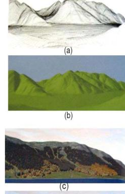
Fig. 7. Computer graphics: a) shows a wireframe rendering of a digital terrain model; b) shows the same landform with solid shading, giving a more easily interpreted result; c) a replanting design rendered more realistically using a more sophisticated modelling system. This uses scanned images of different species of trees; d) shows another version of a design in different weather conditions, illustrating how versatile such rendering systems are. Source: [3]
